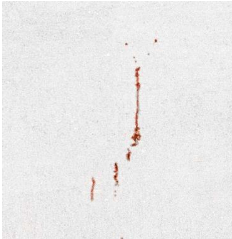
Picture of Red dye penetrant indications
