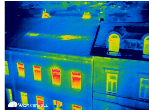
Image courtesy: Workswell Infrared (missing insulation)
