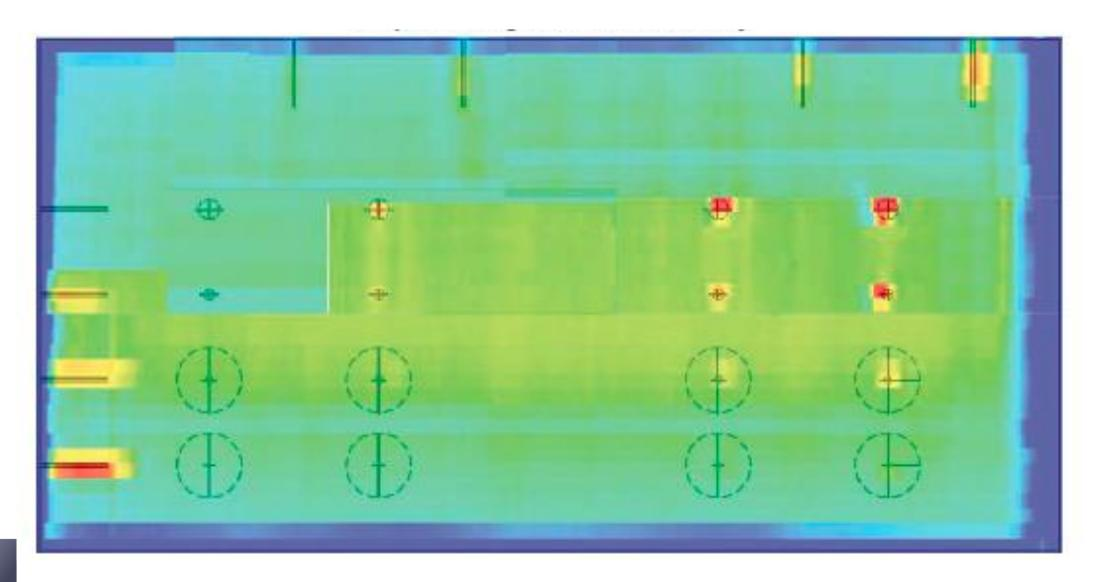
Typical ECA – Low Frequency Probe (Surface Breaking Features)
