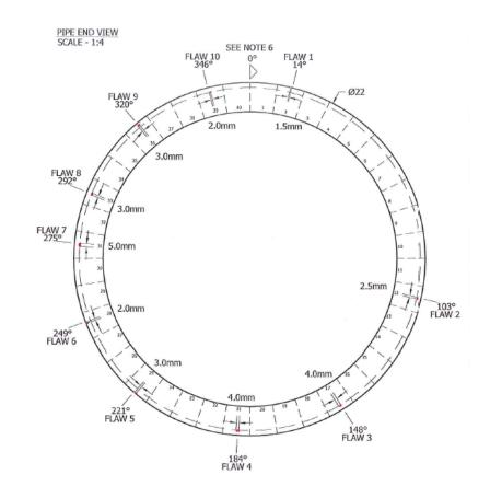
Real Welding Defects (On-Purpose)
