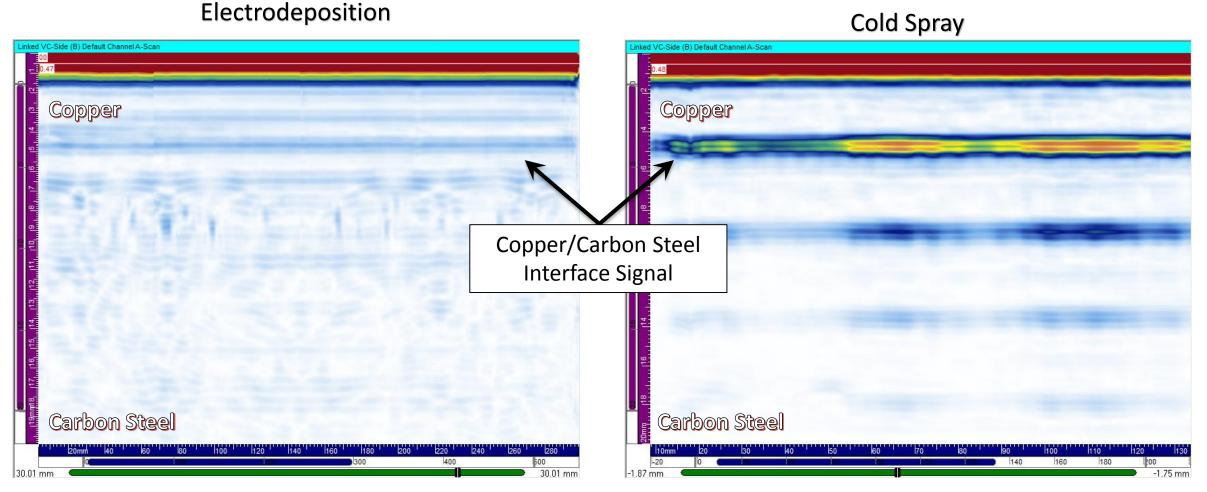
Copper Coating Thickness: ~4.5mm
