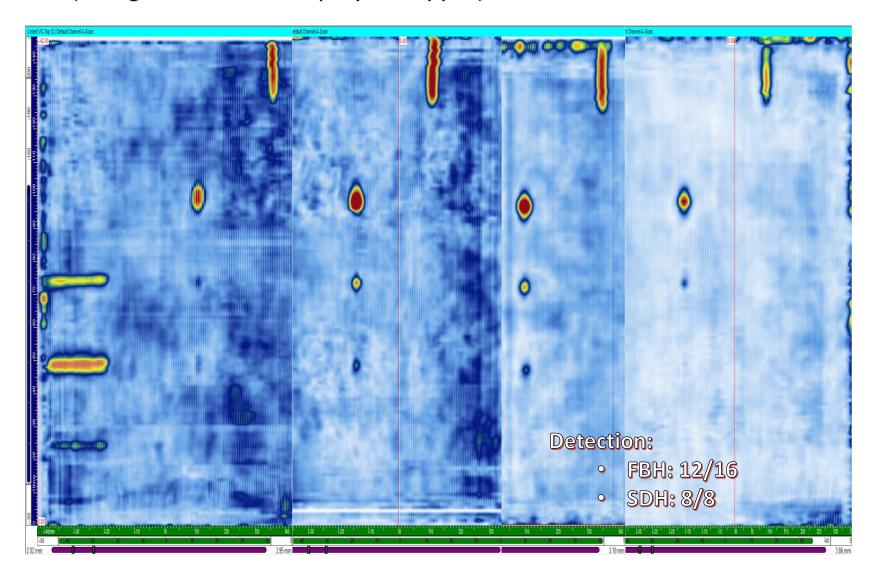
Typical ECA – Low Frequency Probe (In-Volume Features – SDH and FBH)
