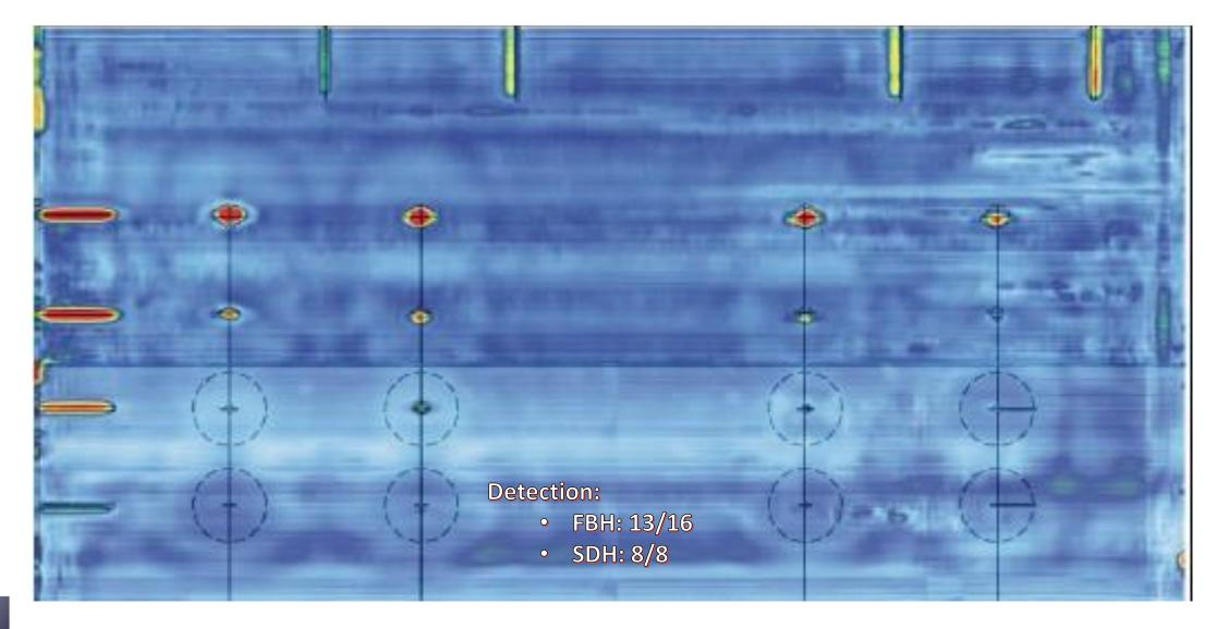
Typical UT Results (Straight Beam - Electrodeposited Copper)
