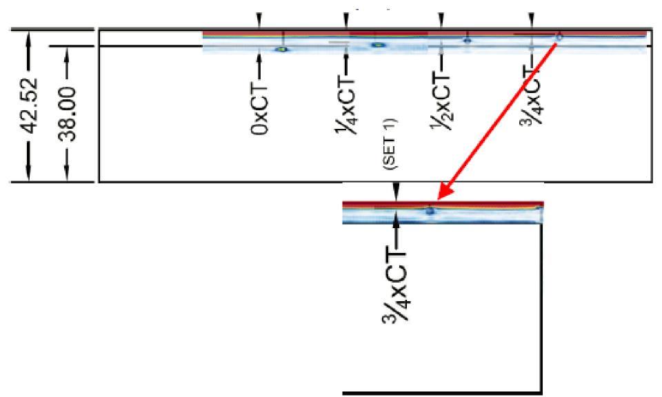
Typical UT Results (Straight Beam - Electrodeposited Copper)
