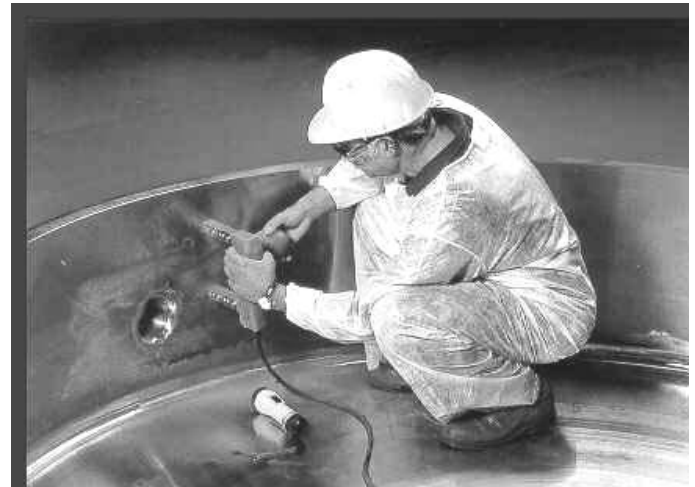
Magnetic Particle inspection using an electromagnetic yoke
