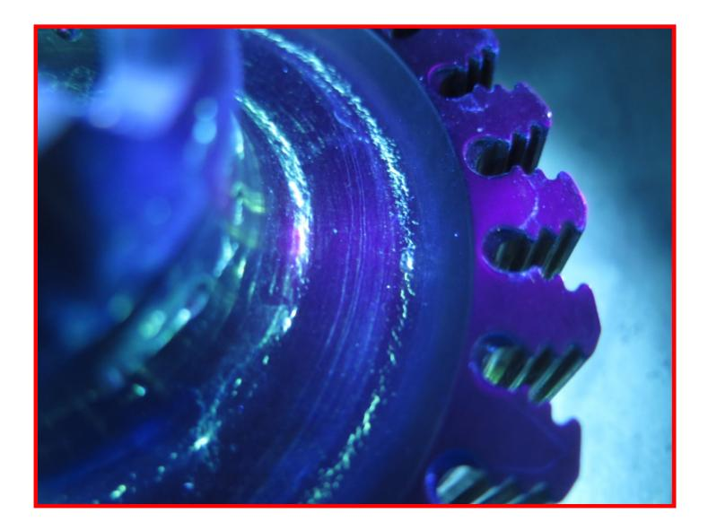
A uncontrolled pre-penetrant etch can result in component failure
