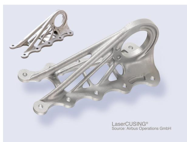
**Bionic cabin bracket** in Airbus A350 XWB built on **M2 cusing /** Material CL 41TI ELI (TiAl6V4 ELI) / Lightweight natural construction solutions can be generated almost 1:1 with the additive LaserCUSING® process. The laser-generated component with an optimized structure delivers a weight saving of more than 30% compared with the component produced by conventional means!
