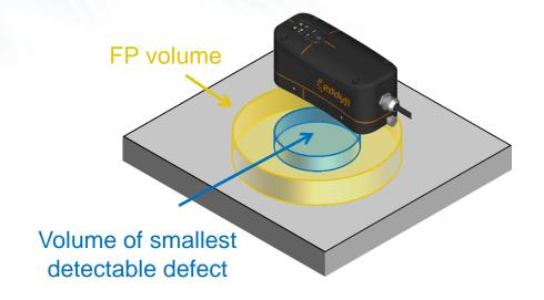
Provide an average WT measurement within the footprint of the probe
