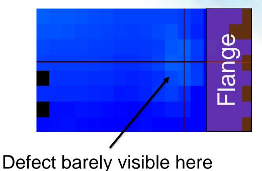
7in OD, STD pipe with small defect milled at 1in from flange
