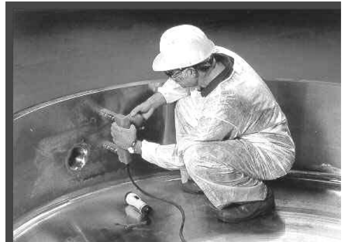
Magnetic Particle inspection using an electromagnetic yoke
